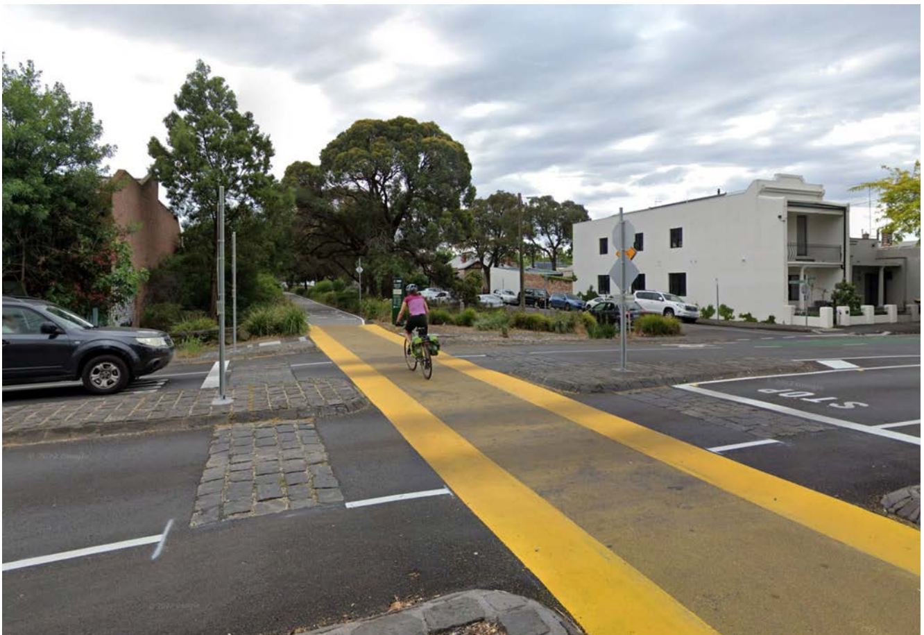
Left: Raised crossing for pedestrians and other active transport modes. Image: Google Street View
