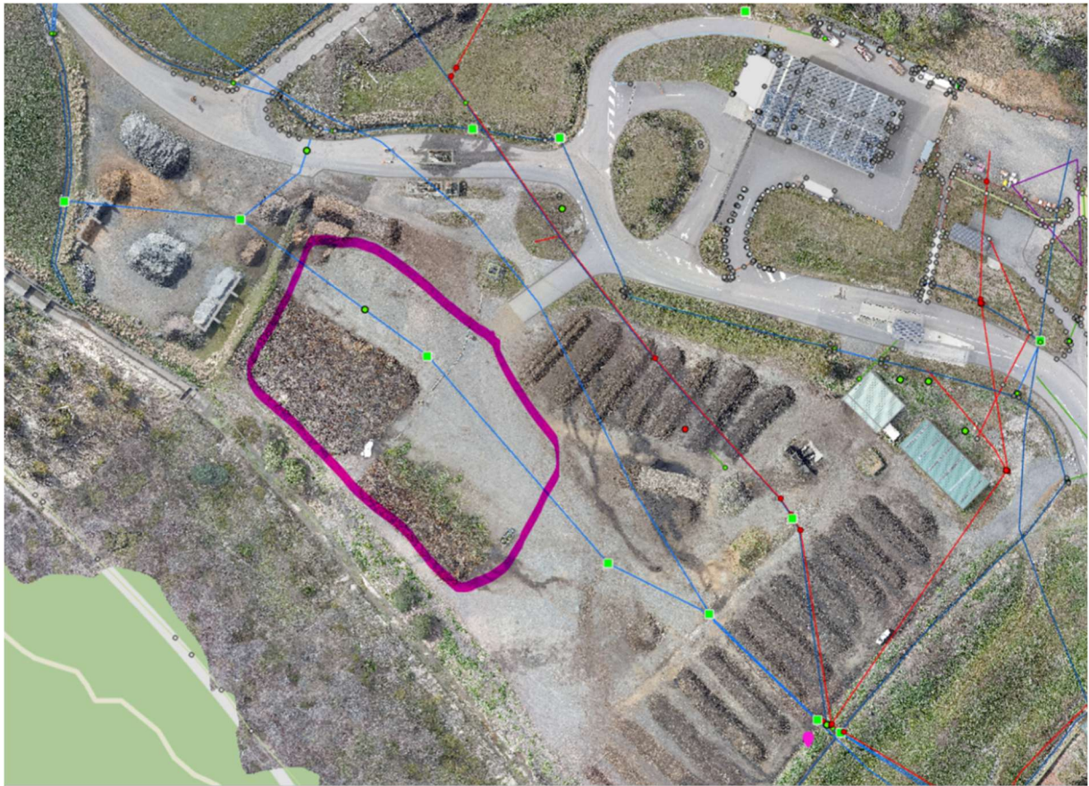
Figure 1. Indicative geofabric repair area within the organics processing area
