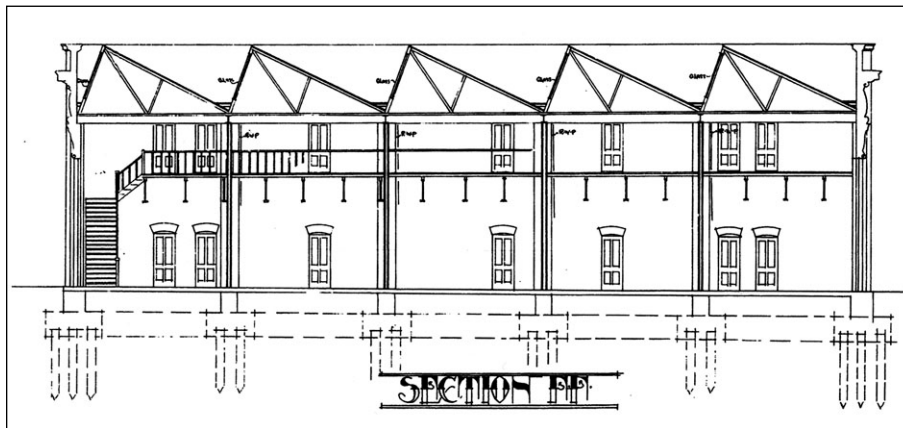
Figure 20. 1914 section showing market entrances to shops and stairs, balcony and doors to storage rooms above the shops. Note also the sawtooth roof and piles below the foundations (HCC Drawing A7 5 ).
