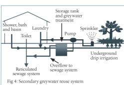
Provided that the required management and maintenance regimes are adhered to, including periodic sludge removal, the effluent should be clear and odourless, and meet health guidelines. Effluent quality should be better than 30 mg/l suspended solids concentration, 20 mg/l BOD5, 0.5 mg/l free residual chlorine and 10 organisms per 100 ml for faecal coliforms. It can then be disposed of by surface
