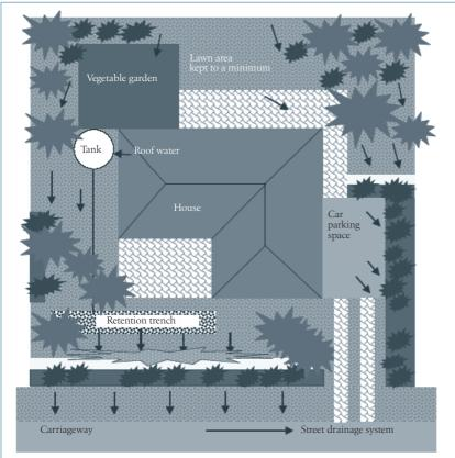
Fig 3: Example of an alternative drainage strategy
