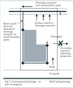
by overland flow. The public drainage system usually consists of a system of gutters, streets, pipes, culverts and channels owned and operated by the local council or other authority.
