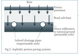
Asphaltic porous paving is laid on a sand/gravel sub-base over natural soil (see Figure 2).
