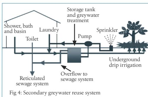
Provided that the required management and maintenance regimes are adhered to, including periodic sludge removal, the effluent should be clear and odourless, and meet health guidelines. Effluent quality should be better than 30 mg/l suspended solids concentration, 20 mg/l BOD<sub>5</sub>, 0.5 mg/l free residual chlorine and 10 organisms per 100 ml for faecal coliforms. It can then be disposed of by surface
