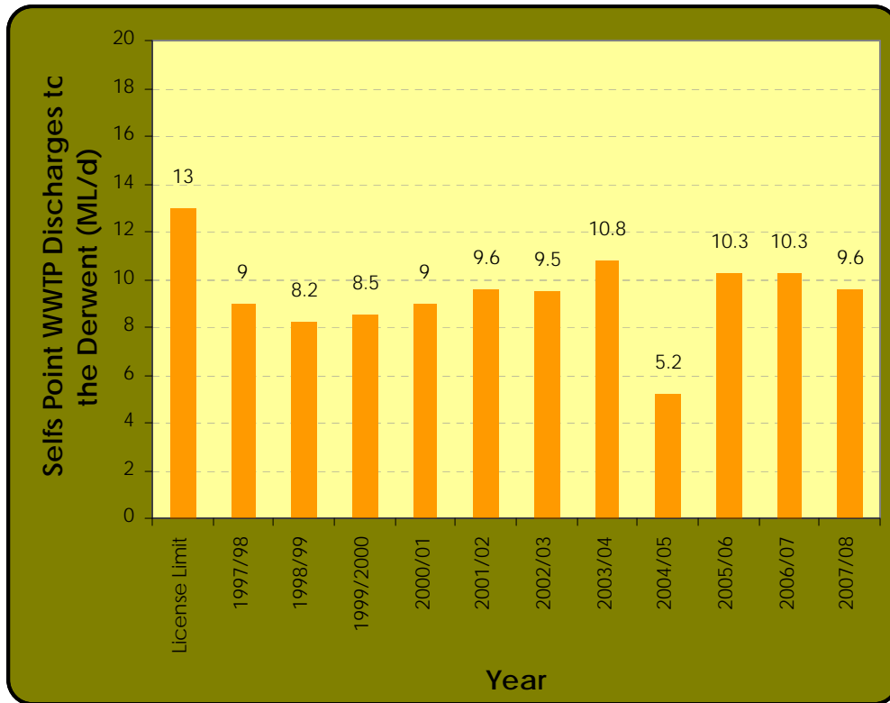
Figure 6-2 Discharges from the Self's Point Waste Water Treatment Plant
