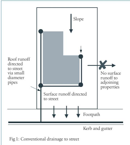
convey stormwater to the street drainage system with a minimum of nuisance, danger or damage. Roof runoff is discharged via small diameter pipes (usually 100mm diameter), and surface stormwater is usually conveyed
