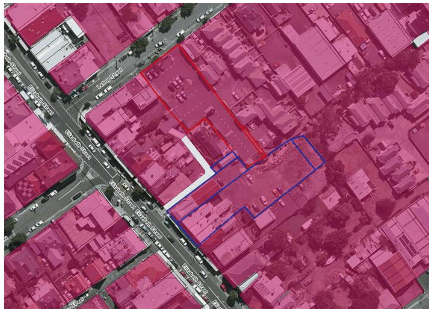
Figure 2: Subject site (outlined in blue); Council Lefroy Street carpark (outlined in red); showing land serviced by TasWater reticulated sewer infrastructure (light marone); Right of Carriageway providing access from Elizabeth Street shown in solid white.
