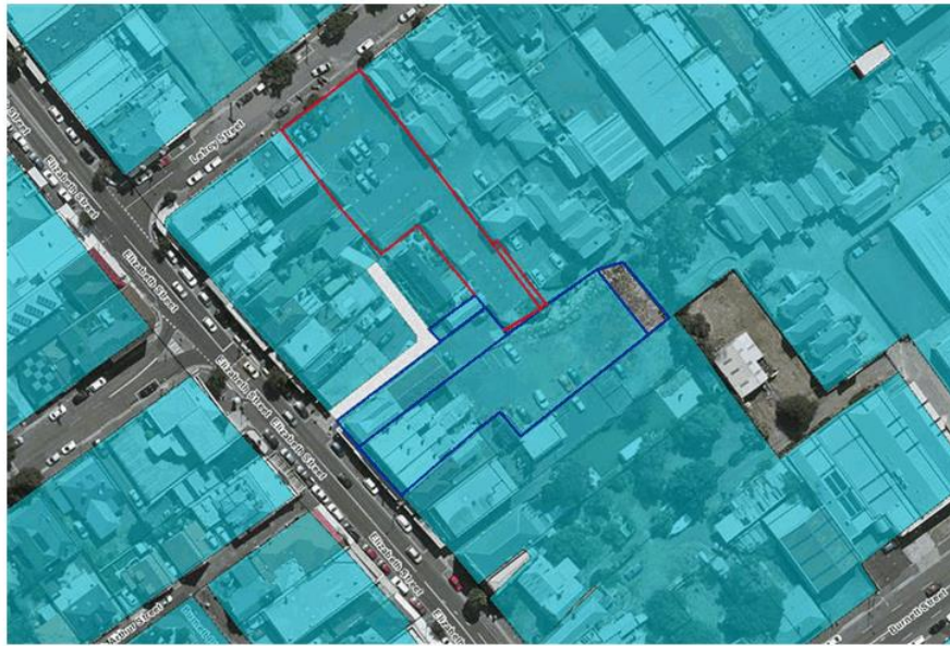
Figure 1: subject site (outlined in blue); Council Lefroy Street carpark (outlined in red); showing land serviced by TasWater reticulated water infrastructure (light blue); Right of Carriageway providing access from Elizabeth Street shown in solid white.
