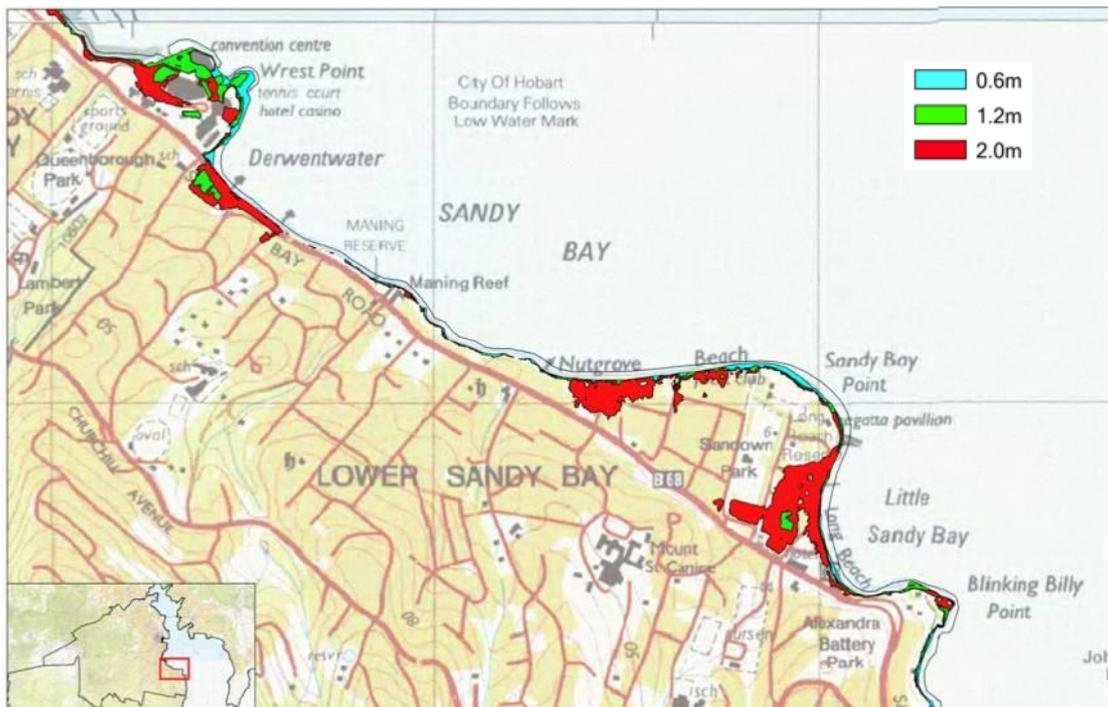
Figure 4: Sea level rise inundation mapping for Hobart's municipal area for the year 2100
