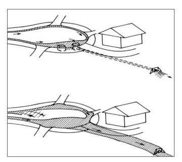
The stormwater network operating as designed: in small to moderate rainfall events, runoff is contained within kerbs and the piped system. In extreme events, runoff will follow overland flow paths.
